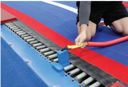
**Step 3:** Attach the non ratchet end of the strap into Bracket #1. Failure to attach properly could result in injury.
