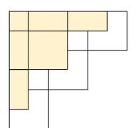
Continue to add panels (expanding out from the original corner) with great attention to abutting the panels and keeping them square. All the edges should align. (Adding the top layer as you work across will keep the panels from wandering.)
