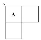
Bottom panels have blue velcro on top, springs on bottom. Start in <u>one</u> corner with three bottom (springed) 5' x 5' panels. (Do not start at each corner and work toward center.) Carefully align the edges to be squared up.
