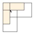
Apply the top layer as shown, starting first with the one  $2\%' \times 2\%'$  panel and then the two 5' x 2%' panels. This secures perfect alignment of the bottom. (To maintain alignment, be careful not to walk on the unsecured bottom panels.)
