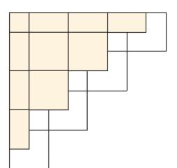
Refer to the layout when you get to the far edges. Some mild warping may occur as a result of banding for shipment. Generally the velcro will hold the boards in place, especially when it is covered with a foam product. In worst cases, you might have to temporarily place a weight on the offending panel or put a screw in the panel until the warp disappears. You are now ready to roll out your Carpet Bonded Form or Flexi-Rolls. We thank you for your purchase.
