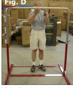
\*If the Bar Assembly is difficult to move, raise and lower several times. This will free the chambers of any extra paint or metal particles that may have been stuck in the chamber during the manufacturing process.
