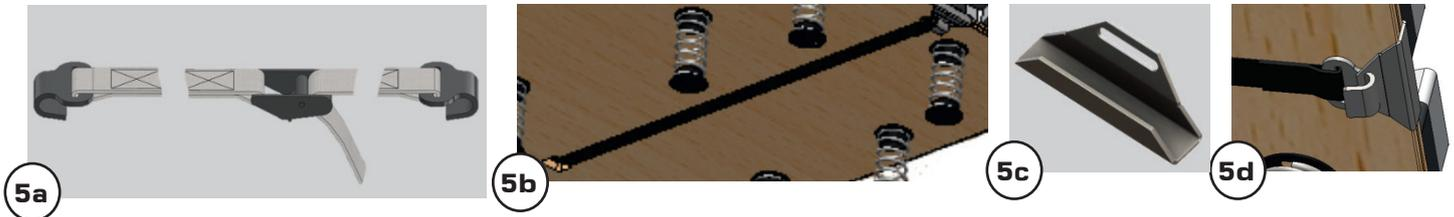
Combine a long and a short tension strap at the buckle (pict. 5a) - as a final result there have to be 25 tension straps.
