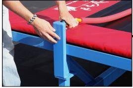
Attach the end of the strap with the ratchet to Bracket #2. Remove the PTO pin and open the hinged bracket. Slide Bracket #2 on to the opposite leg, placing it tightly against the leg. Close the hinge and replace the PTO pin into the hole. Begin to tighten the ratchet. You will want to push down on the bracket to make sure it is tight to the Tumbl Trak.
